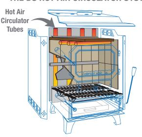
Vertical tubes in the firebox increase the heating surface area by approximately 50%. Heat rises inside the tubes, drawing cooler air from the floor. This convection process produces circulation with no need for electrical blowers or fans, meaning even heat throughout your home.
