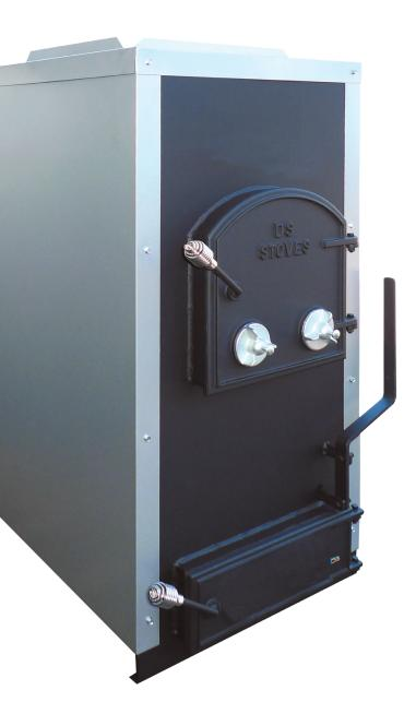
All units require a Class "A" all fuel chimney. Installation must conform to state and local codes. The Ecomiser was designed to be economical. This U.L. Tested anthracite burning furnace is controlled with a DS Hot Air Draft Regulator, combining with a reburn system for maximum efficiency using less fuel. The Ecomiser offers a domestic water option and a single-speed blower. It can heat a whole home, shop, or greenhouse for less money.
